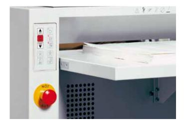
**FOLD-AWAY FEEDING TABLE** The fold-away feeding table is ideal for inserting flat paper. A photo cell automatically starts and stops the cutting head when using this feed opening.
