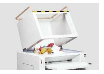
**FEEDING HOPPER** Should a paper jam occur, the electronically secured feeding hopper can be tilted for safe and convenient clearing.
