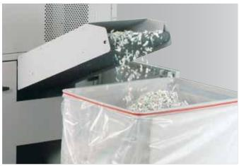
**CONVEYOR BELT SYSTEM** By using the conveyor belt system the output of the shredder can be doubled (removing of the full plastic bag is not necessary).
