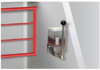
**EASY LUBRICATION** A centralised oiler for easy lubrication of the cutting head is standard equipment on this high-capacity shredder.
