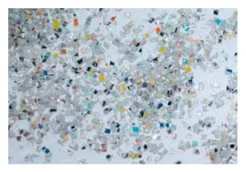
**PARTICLE SIZE 2.2 X 4 MM** Each CD or DVD is turned into approx. 1,200 small particles of 2.2 x 4 mm in size. The picture shows the original particle dimensions.
