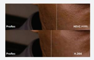
Compared with H. 264, the greatest strength of H. 265 is that it has a higher compression ratio, which can be discerned from its name. H.265 is also called HEVC (High Efficiency Video Coding), and the primary use is to further reduce the design flow rate, in order to lower the cost of storage and transmission.
