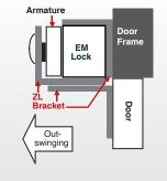
Mounting with "ZL Bracket " for in-swing door application.
