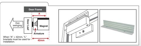
Adjustable "L" bracket for outward door when the header is narrow.
