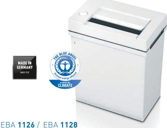
Automatic start/stop controlled by photocell. Automatic reverse and power cut-off in case of overfeed. 220 mm feed opening. Quiet, 150 watt single phase motor. Double motor protection against overheating. Magnetic safety switch cuts power to motor when shredder unit or bin is removed to
