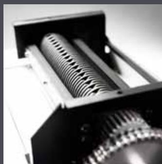
Specially hardened HSM cutting rollers ensure absolutely precise cutting.
