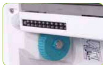
See-through sensor (Auto Detection)
